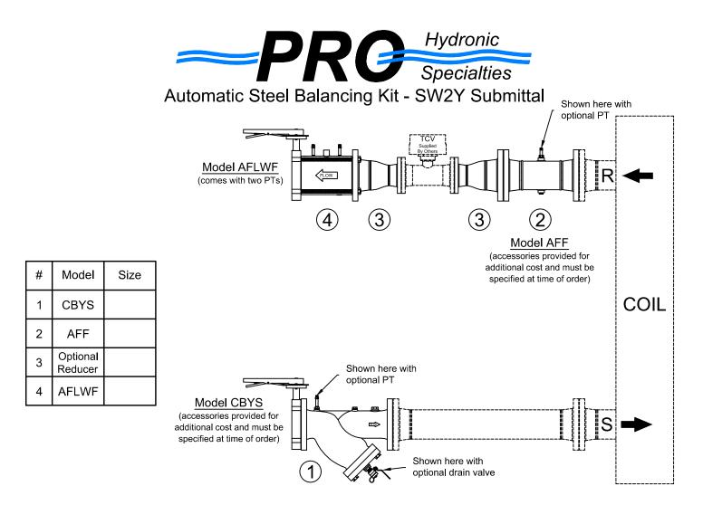
**PRODUCT DESCRIPTION:** The Automatic Balancing Valve Kit is a packaged and partially preassembled grouping of components required to complete installation of a terminal unit. Temperature control valves, piping, and coils are supplied "by others". Mounting and testing of the customer provided TCV is available at an additional charge. Parts for reductions in line size are available for an additional charge. Consult with factory for information and pricing.
